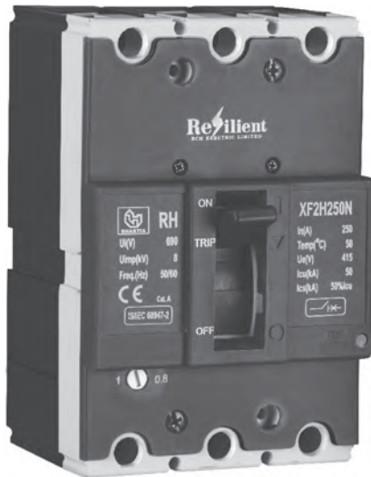
Frame -2 : I cu /I cs = 25/25, 36/18, 36/27, 36/36, 50/25, 50/50 kA
